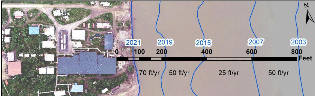
**Figure 1.** Kuskokwim River shorelines (blue) in relation to the school. The image is from the June 29, 2021 drone survey. The average erosion rate from 2003 to 2021 is 40 feet per year. Recent rates are 50 to 70 feet per year. The school is 79 feet from the bank and about 260 feet long.
